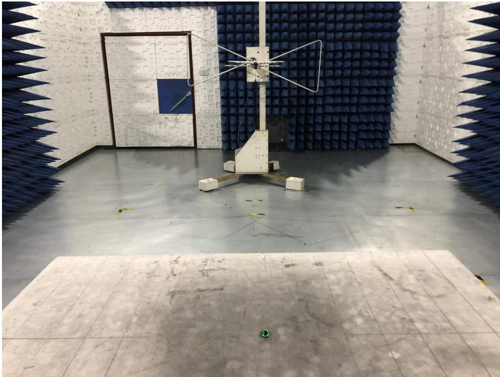
RADIATED EMISSION TEST SETUP ABOVE 1GHz
