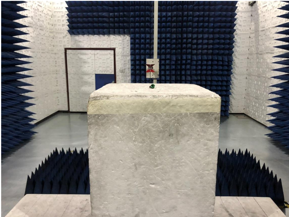
RADIATED EMISSION TEST SETUP ABOVE 1GHz
