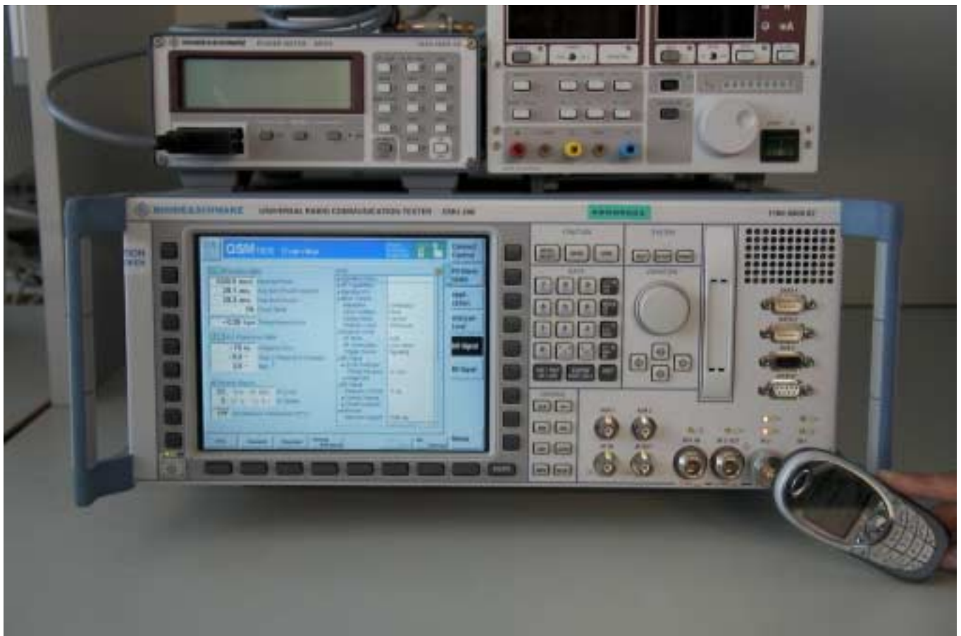
Fig. 2: Set up for conducted power measurement.
