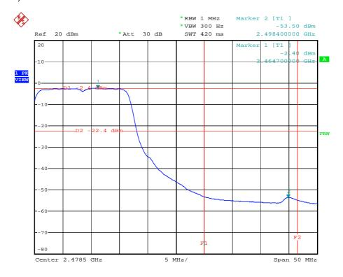
Observation: All emissions in the 100kHz bandwidth are 20dB lower than the carrier strength.
