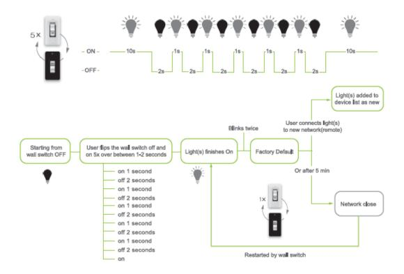
Bulb(s) could be restored to factory default status either by remote controller or by wall switch. Factory default by remote controller is same as un-pairing Bulb(s), while by wall switch is as following.
