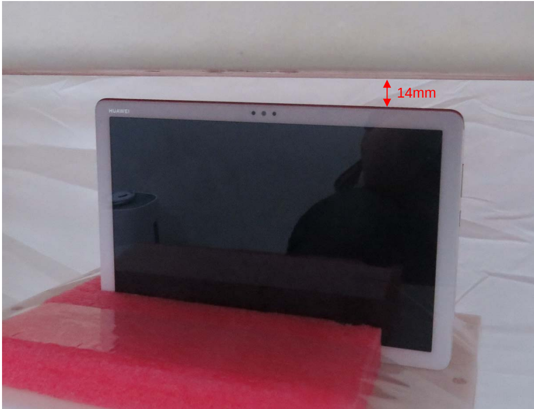
Picture 5: Top Side, the distance from handset to the bottom of the Phantom is 14mm
