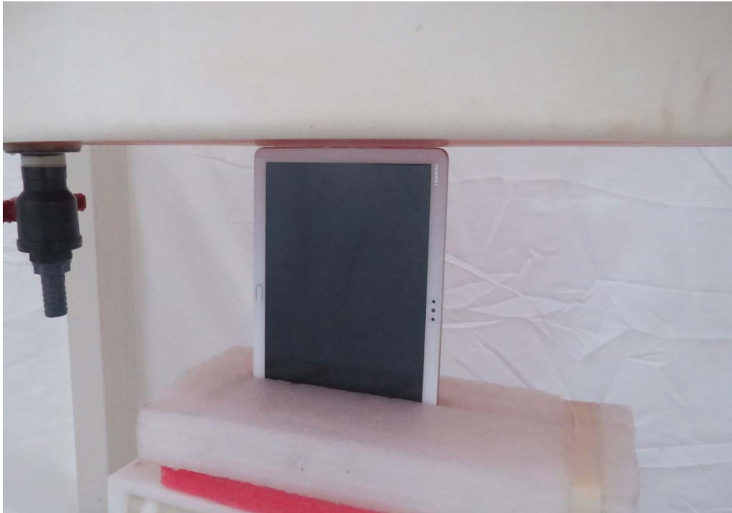
Picture 3: Left Edge, the distance from handset to the bottom of the Phantom is 0mm
