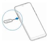
Pull out the card tray and place a nano-SIM card in slot 1 and a microSDXC card (optional) or a nano-SIM card in slot 2, as shown. Carefully slide the tray back into place.
