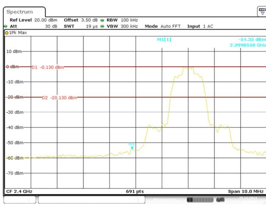
**EDR ( $\pi/4$ -DQPSK): Band Edge-Right Side**
