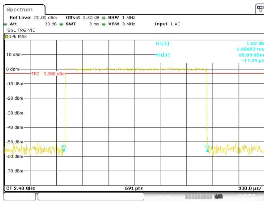
**Pulse time, Low Channel, DH5**
