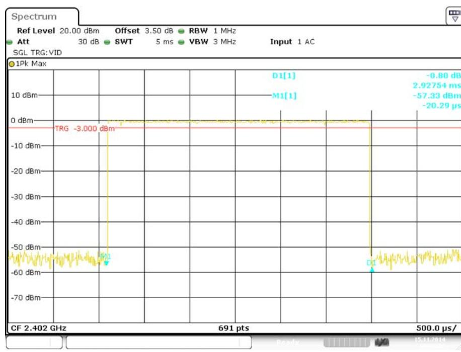
**Pulse time, Middle Channel, DH5**
