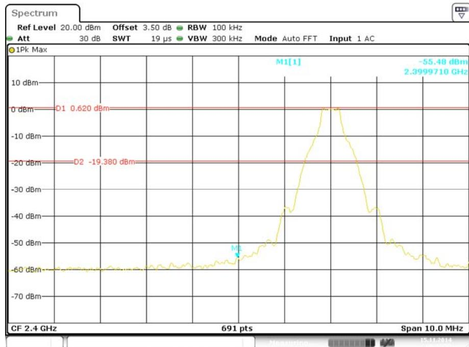
**BDR (GFSK): Band Edge-Right Side**
