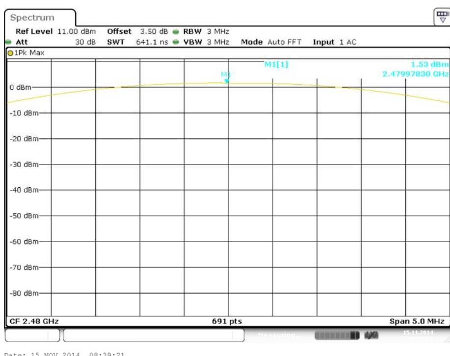
**EDR( $\pi/4$ -DQPSK): Low Channel**
