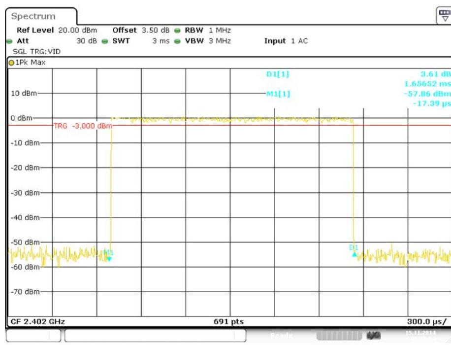
**Pulse time, Middle Channel, DH3**
