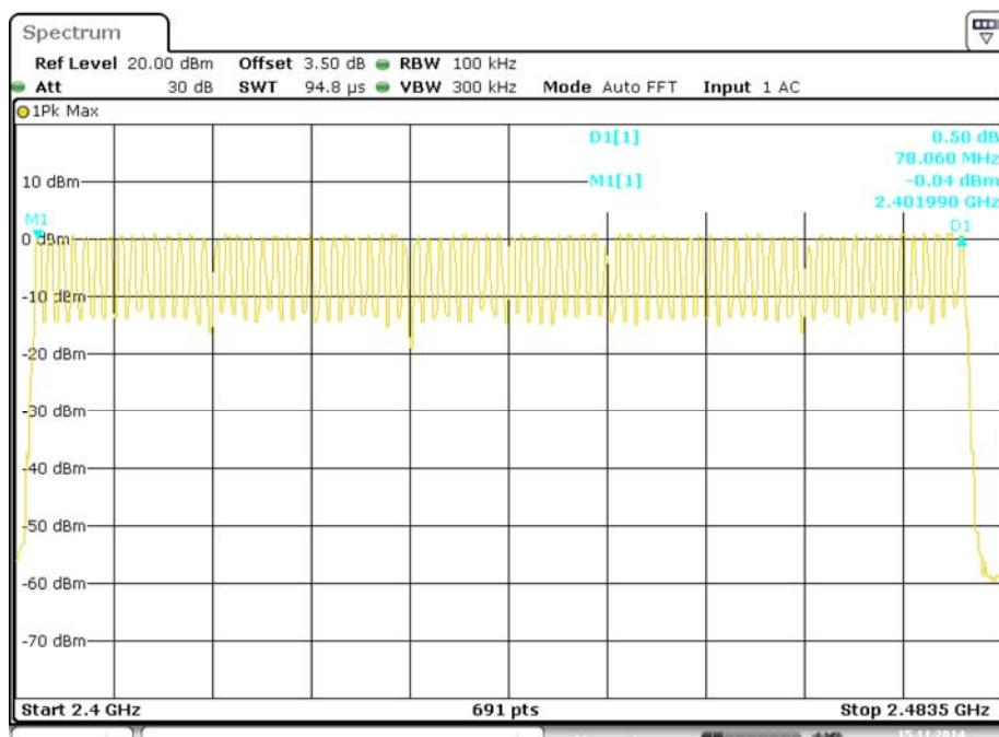
**EDR ( $\pi/4$ -DQPSK): Number of Hopping Channels**
