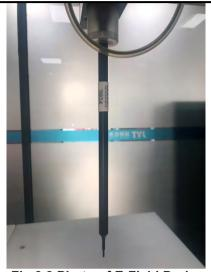
Fig.8.2 Photo of E-Field Probe
