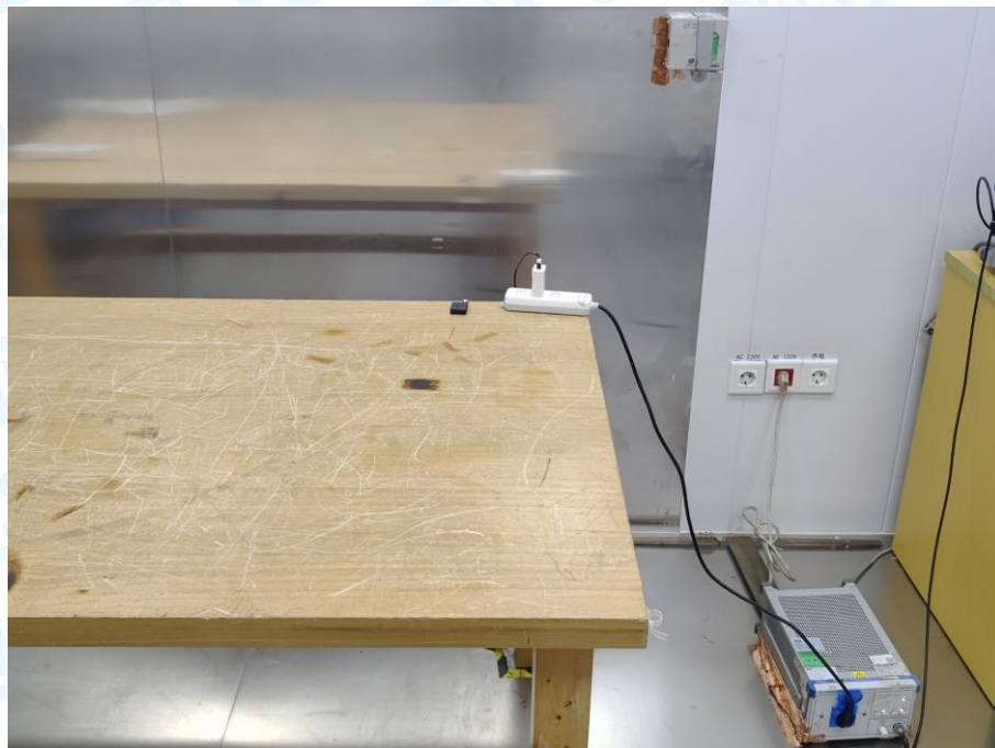
Photo of Setup for Conducted Emission
