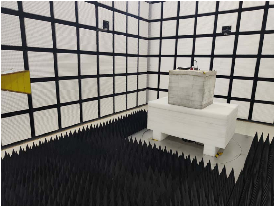
Radiated Emissions Above 1G View
