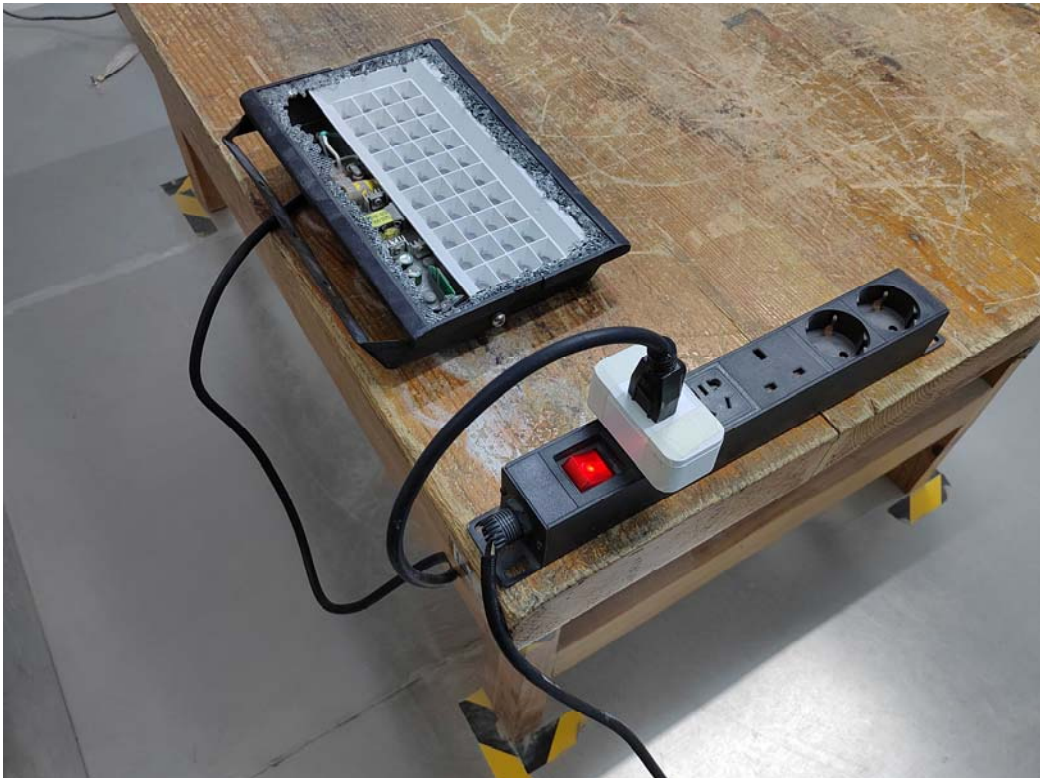
Conducted emissions side View
