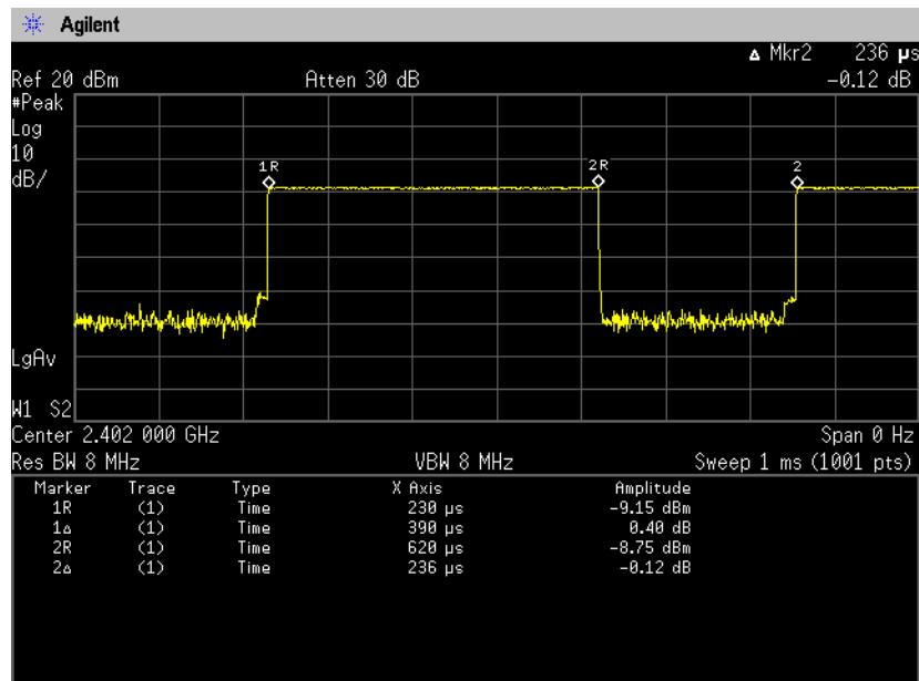
$$\text{Duty Cycle} = T_{\text{on}} / (T_{\text{on}} + T_{\text{off}}) = 390[\text{us}] / (390[\text{us}] + 236[\text{us}]) = 62.3[\%]$$
