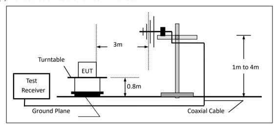
(c) For radiated emissions above 1000MHz
