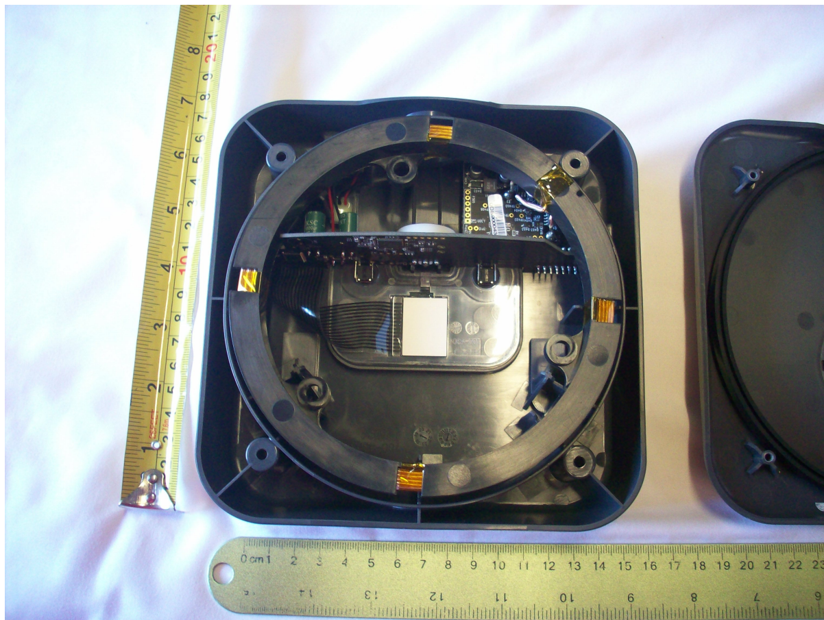
Figure 3. All Models, PCB Close-Up Overview
