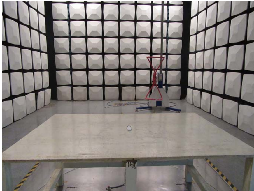
Radiated Disturbance Test Setup View (Below 1GHz)
