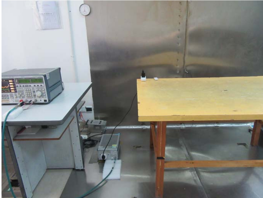
Conducted Emission Test Setup Front View
