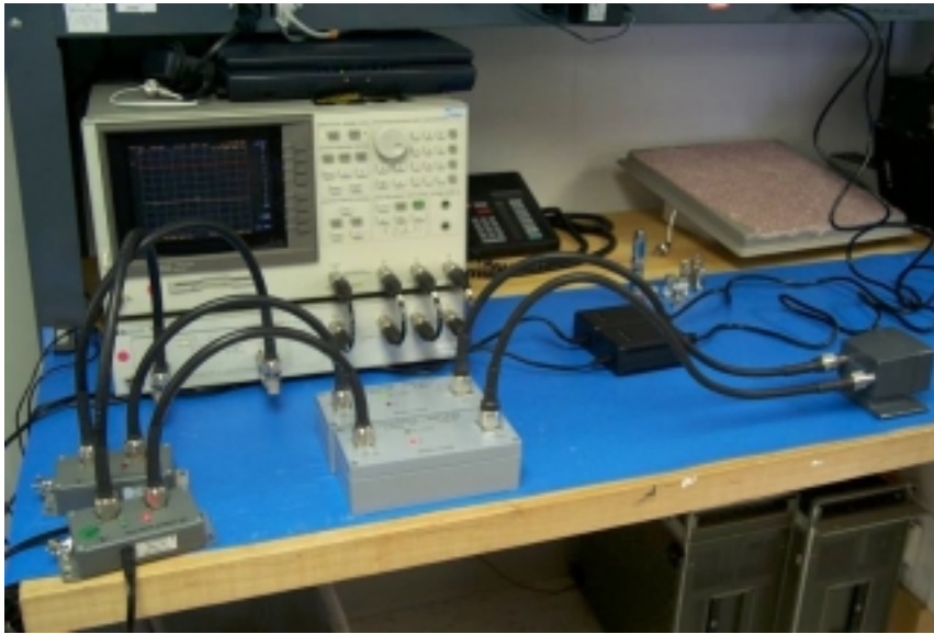
Figure 8 – Linearity of Conversion 2.4 -> 5.8 -> 2.4 GHz Verification
