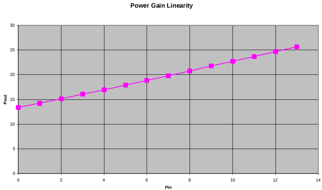
Figure 6 - Power Gain Measured Linearity
