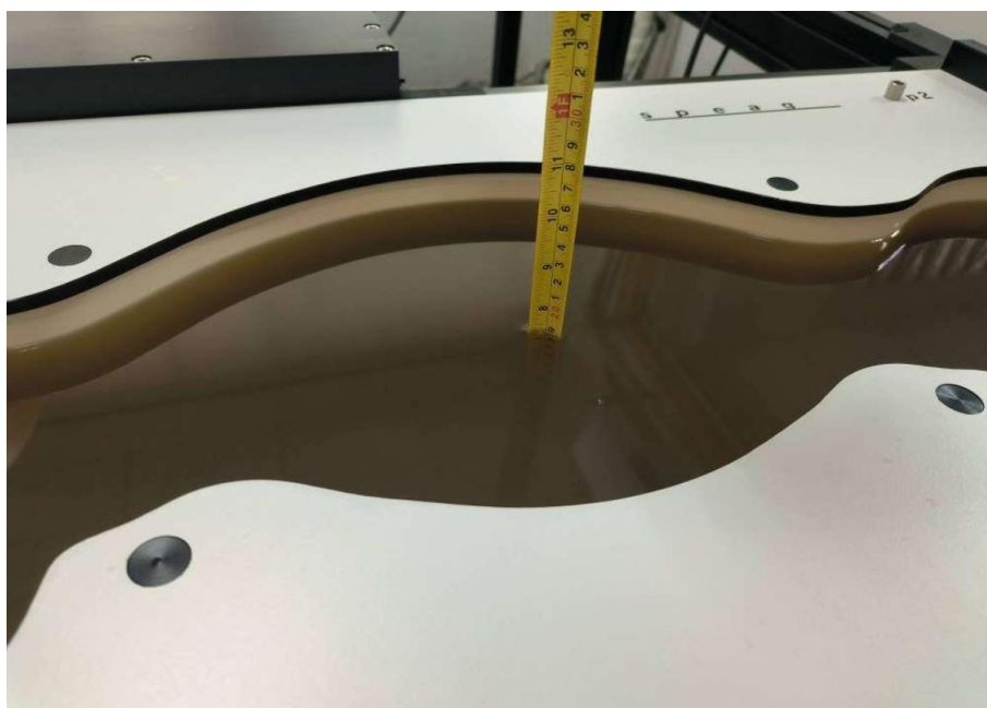
Picture 7.2 Liquid depth in the Flat Phantom (0.6GHz - 7.5GHz)
