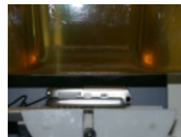
Figure A.5 Body SAR Test Setup -- w/o Belt Clip --
