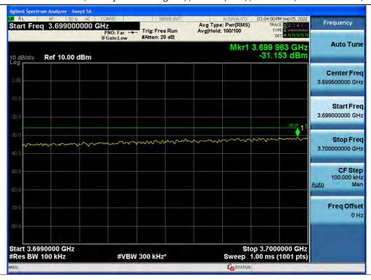
+3 dB above Out-of-band (two adjacent test signals) / C-Band(Ant1) / Downlink / 5G NR 100 MHz / Upper
