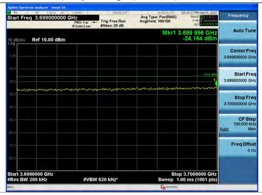
+3 dB above Out-of-band (two adjacent test signals) / C-Band(Ant2) / Downlink / 5G NR 20 MHz / Upper
