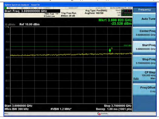
+3 dB above Out-of-band (two adjacent test signals) / C-Band(Ant2) / Downlink / 5G NR 40 MHz / Upper
