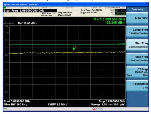
+3 dB above Out-of-band (two adjacent test signals) / C-Band(Ant1) / Downlink / 5G NR 40 MHz / Upper
