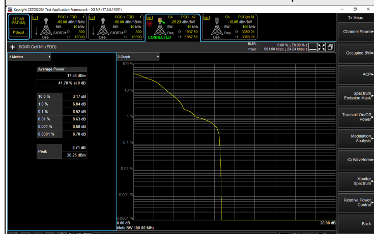
256QAM CH 371500 (1857.5 MHz)
