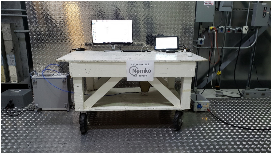
Front Conducted disturbance at mains port setup photo
