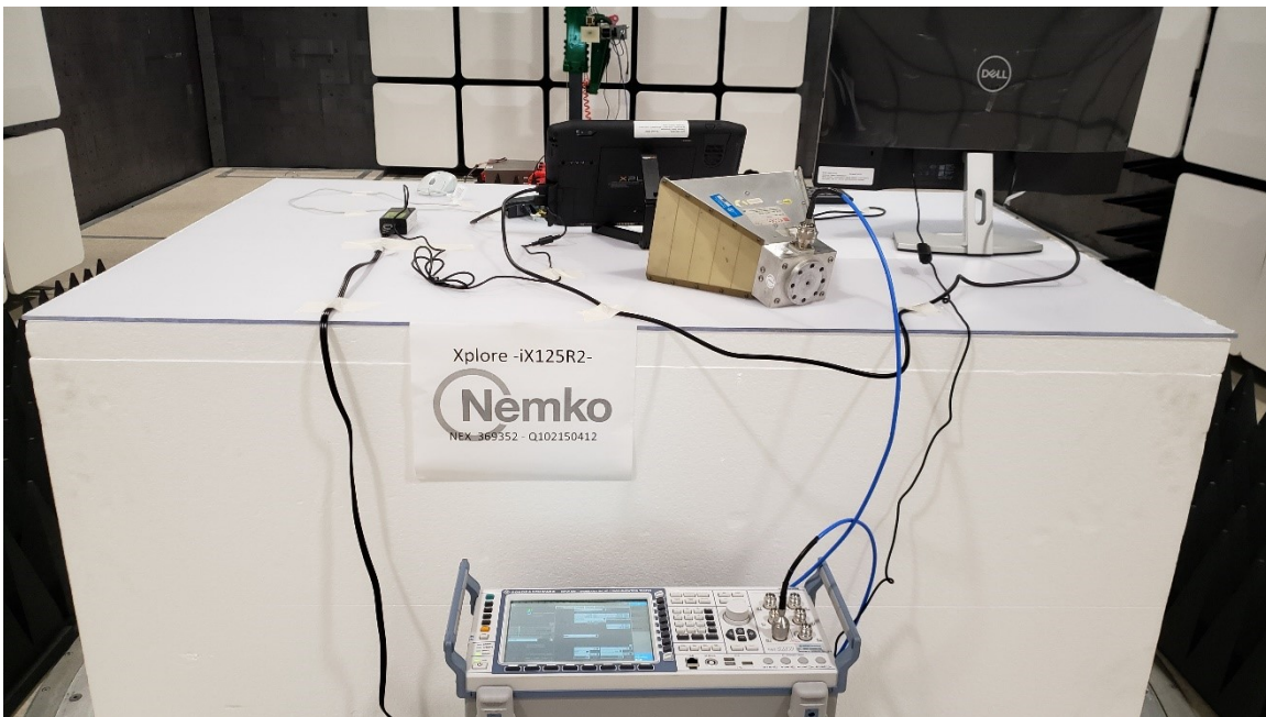
Back Radiated disturbance 18GHz - 26GHz
