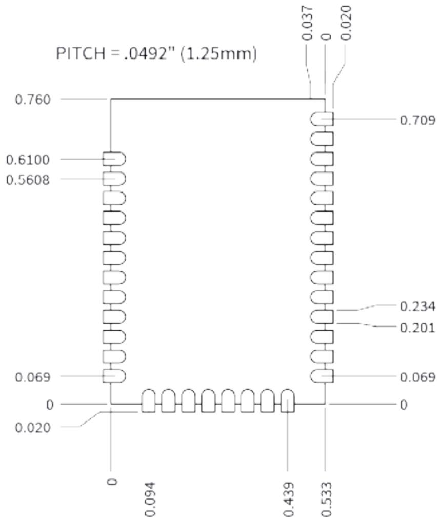
Match the solder footprint to the copper pads, but it may need to be adjusted depending on the specific needs of assembly and product standards. Recommended stencil thickness is 0.15 mm/0.005". Place the component last and set the placement speed to the slowest setting.
