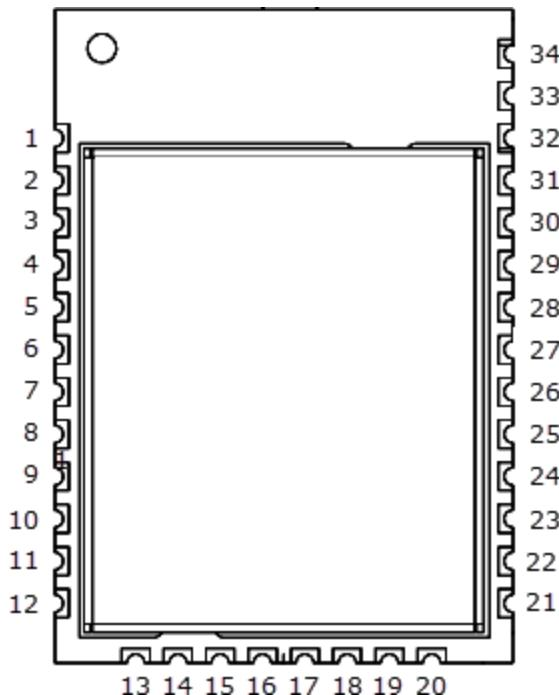
The following table shows the pin signals and their descriptions for the XBee RR RF Module.
