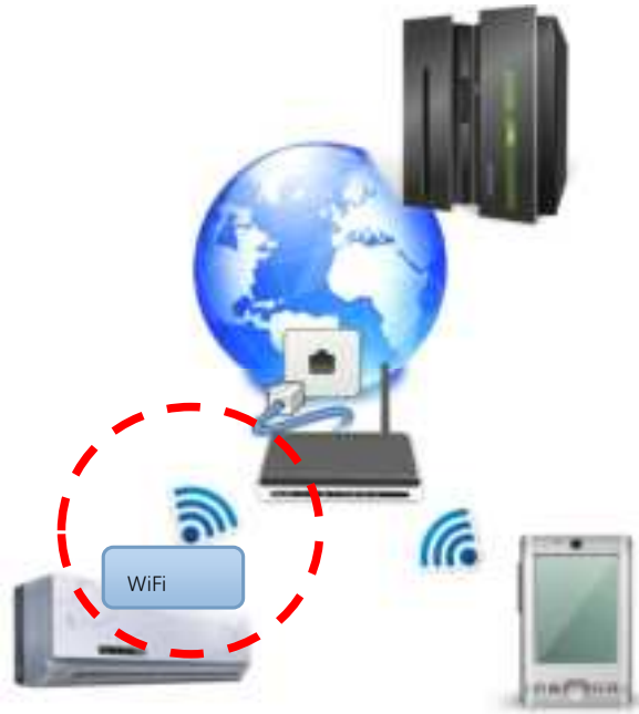
picture 1: The function of WiFi module in the intelligent home appliance system
