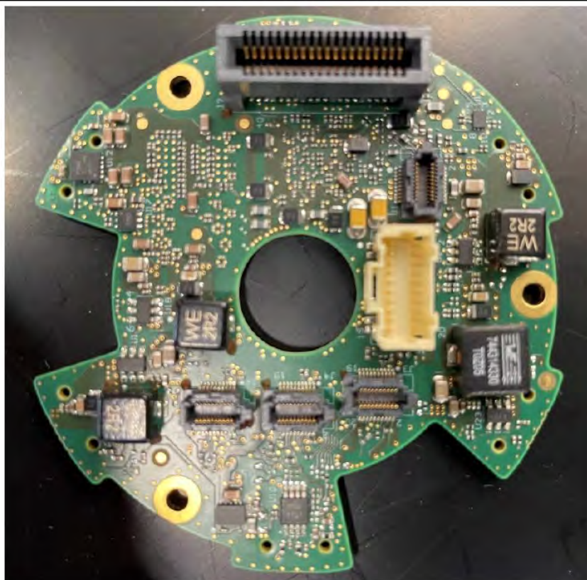
Picture 12: Connection Board Bottom
