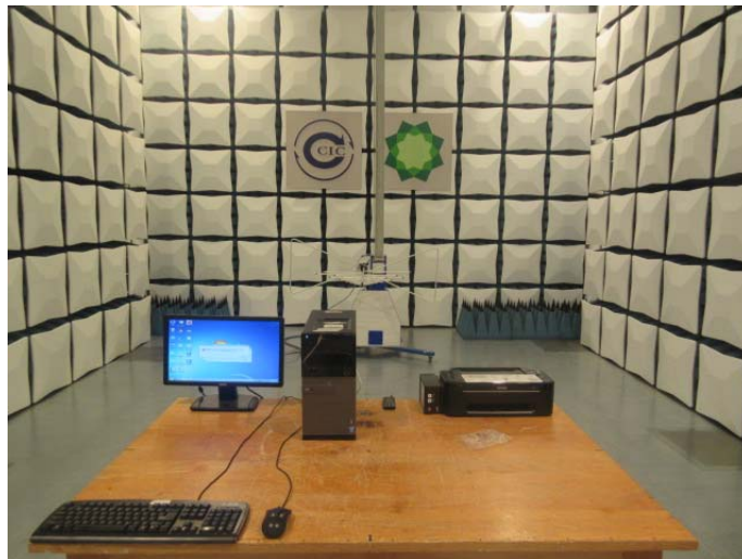
Radiated Emission (above 1GHz) Connect to PC
