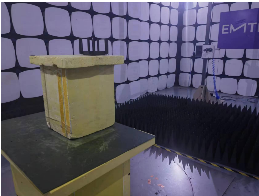
Spurious Emission Test Setup (Above 1GHz)
