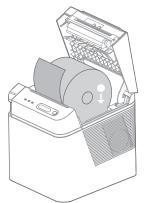
Press the door cover button to open the printer flip cover.
