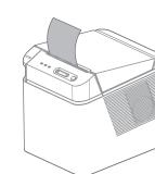
Cover the printer flip cover (Note: When printing blank, please make sure that the paper roll is installed in the correct direction)
