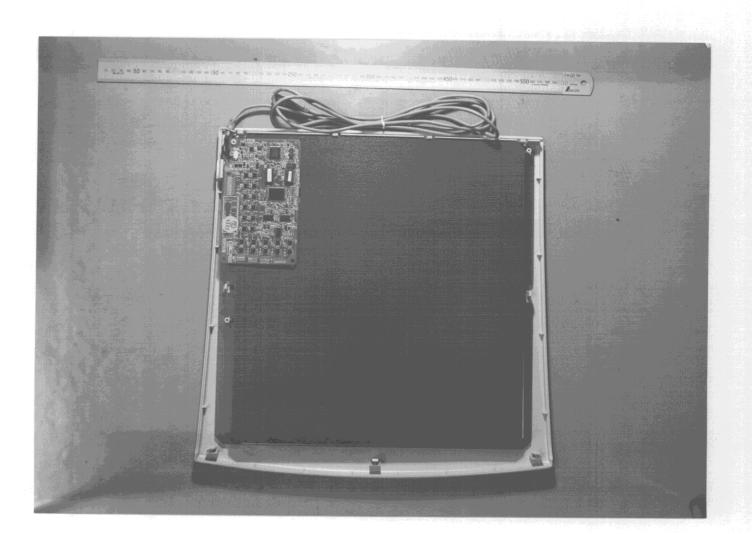
${\tt General-Shows\ front\ view\ of\ P.W.B\ for\ Sensor\ Board.}$
