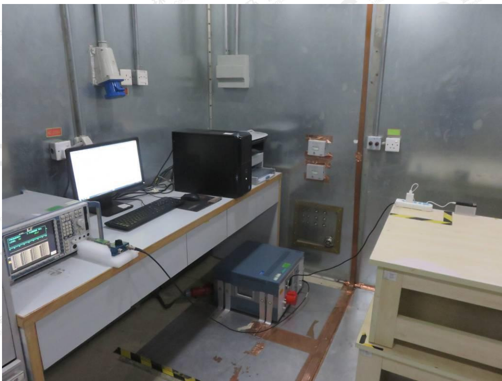
FCC RADIATED EMISSION TEST SETUP
