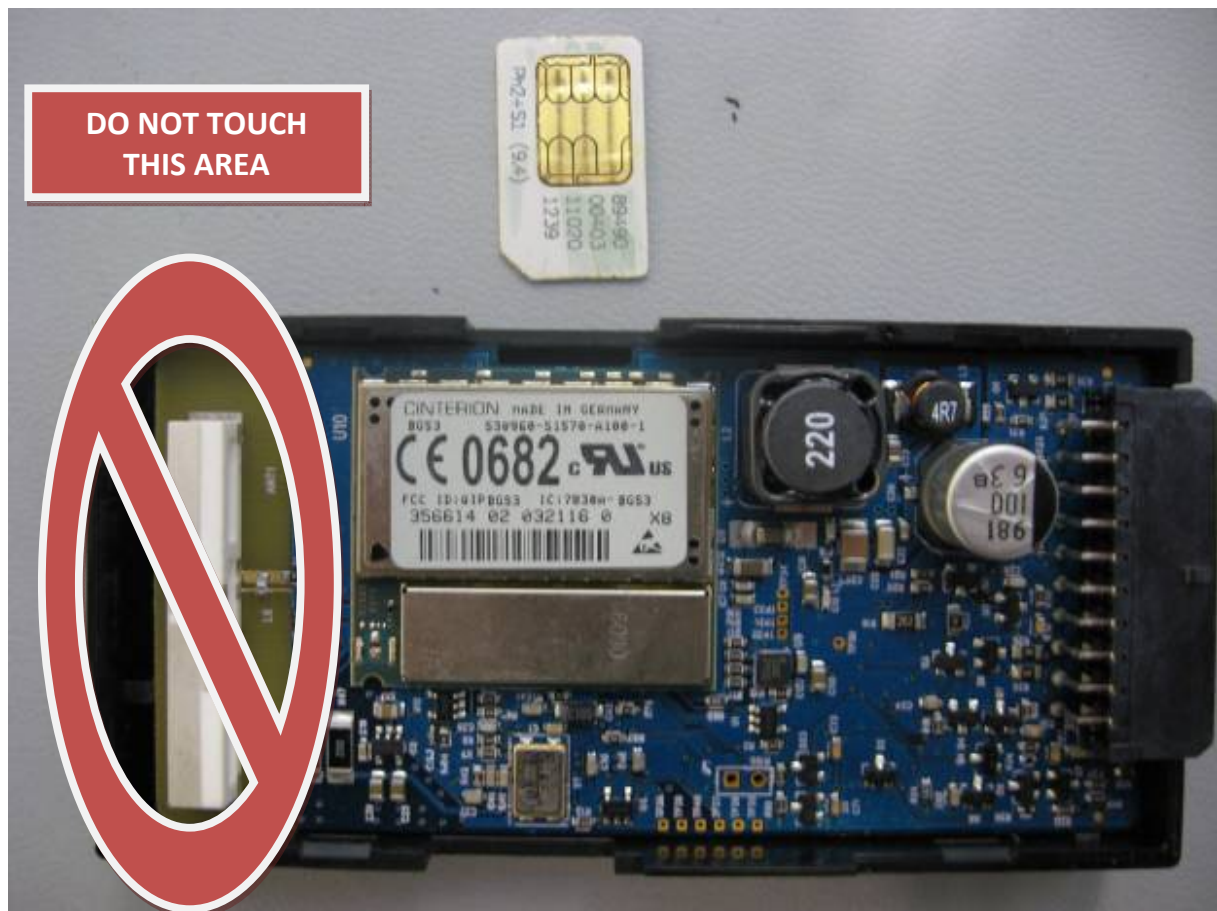
Figure 12 - LMU-2640™ SIM Alignment
