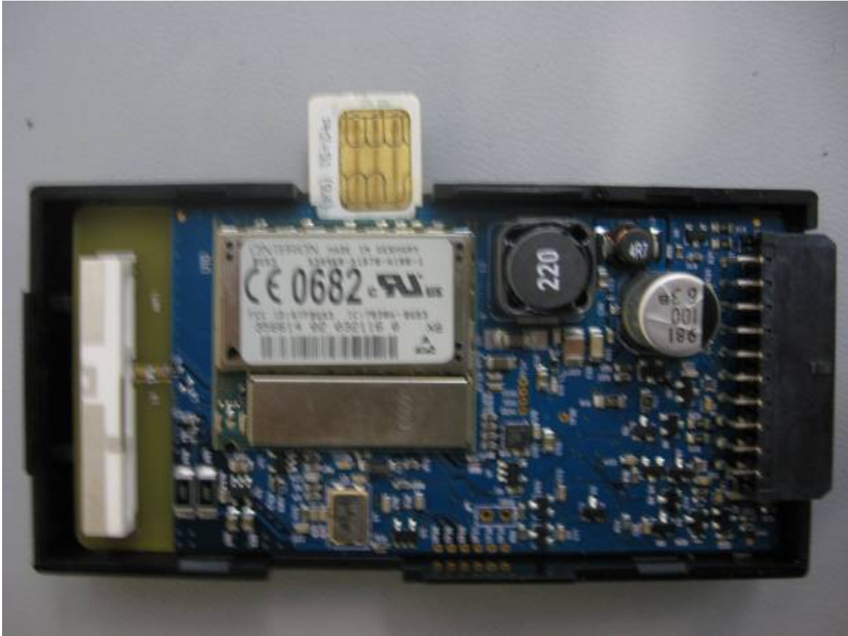
Figure 13 - LMU-2640™ - Partially Inserted SIM
