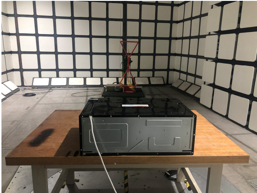
Radiated Emissions - Rear View (30 MHz – 1 GHz)
