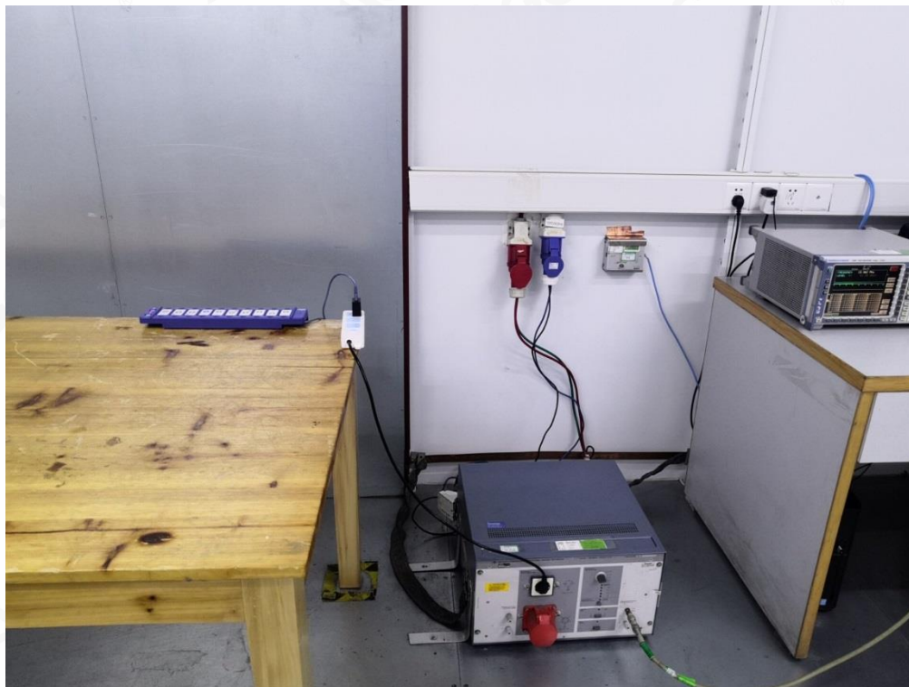
RADIATED EMISSION TEST SETUP BELOW 30MHz
