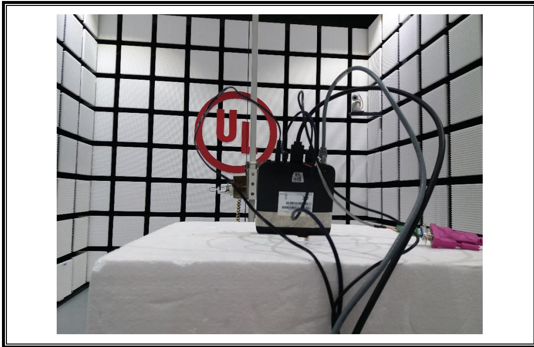
POWERLINE CONDUCTED EMISSIONS MEASUREMENT SETUP-1
