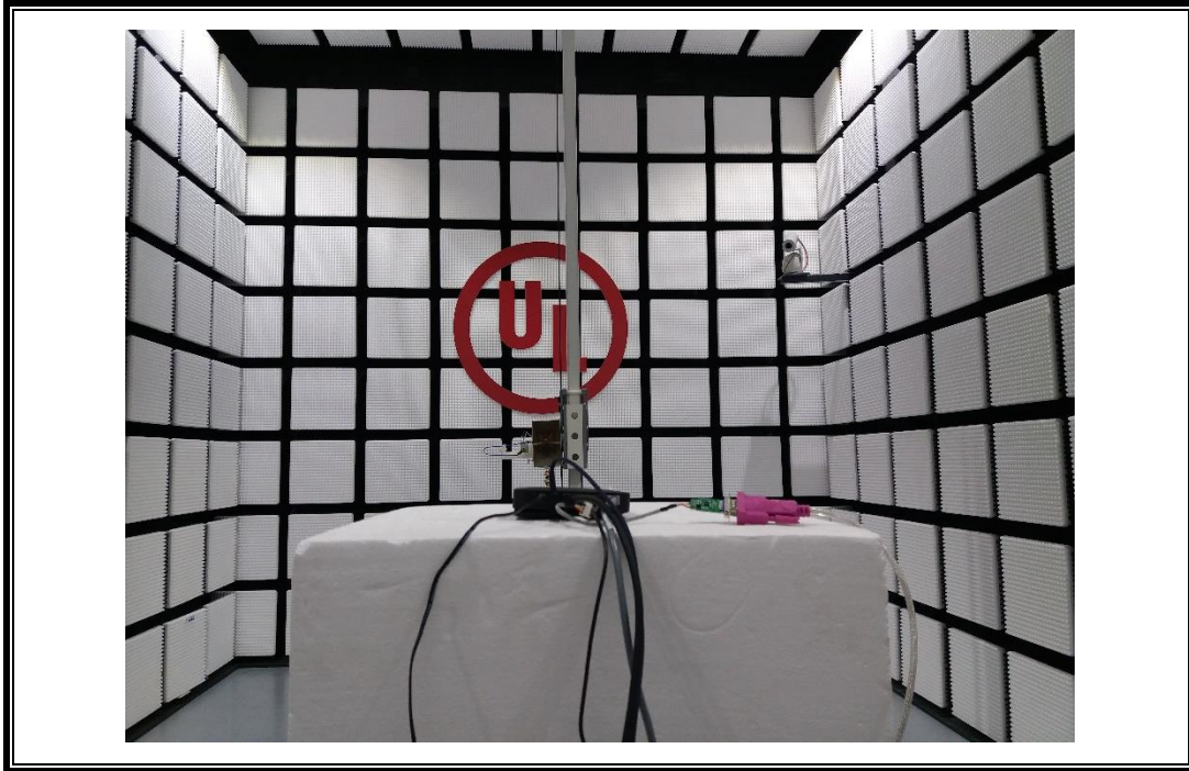
RADIATED RF MEASUREMENT SETUP (X Axis)
