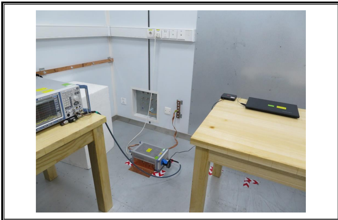
POWERLINE CONDUCTED EMISSIONS MEASUREMENT SETUP-1
