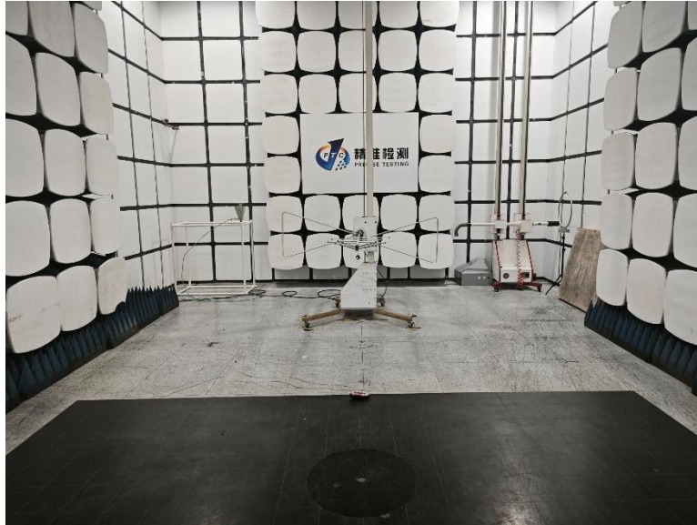
Radiated Spurious Emissions From 30MHz-1000MHz
