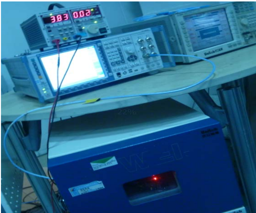
Frequency Stability Under Temperature & Voltage Variations Setup
