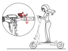
When the scooter starts to move forward, put both feet on the deck and apply the accelerator. (The accelerator initiates once the speed exceeds 3 mph.)
