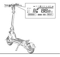
1 Turn the power on and check the battery level indicator.
