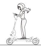
4 Release the accelerator and the kinetic energy recovery system (KERS) initiates automatically to brake slowly; And squeeze the brake lever for a sudden brake.
