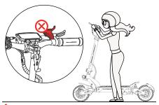
Do not press the accelerator when you're walking the scooter.
