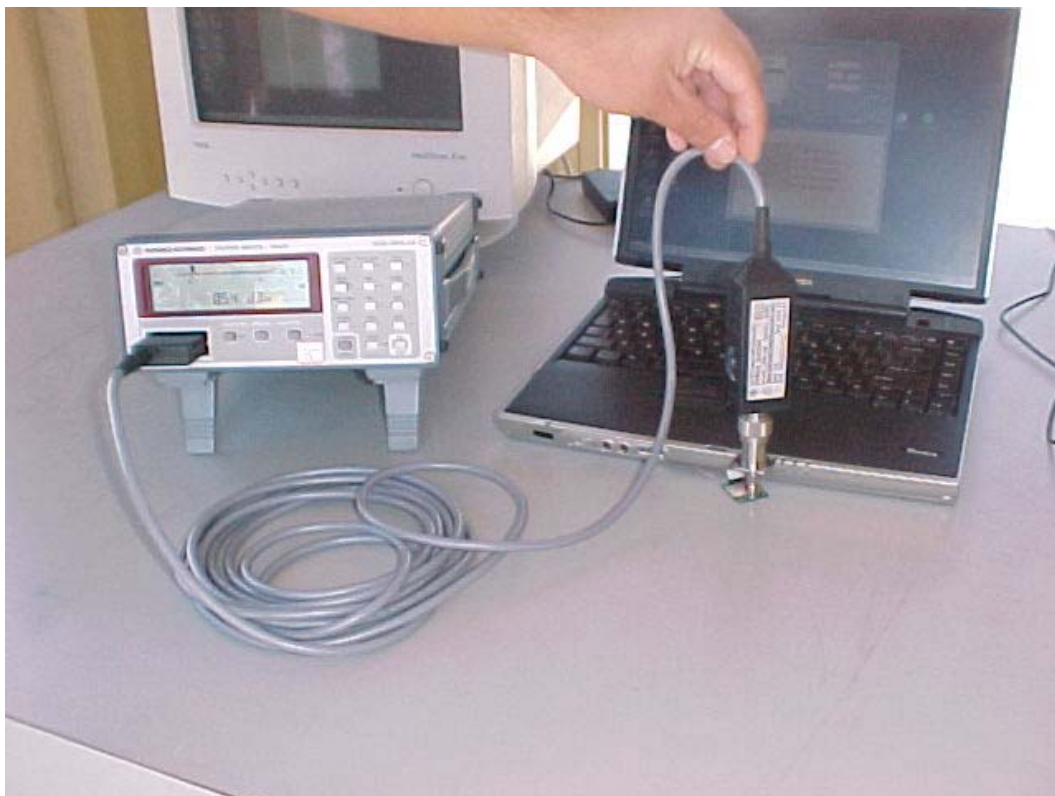
Maximum Peak Output Power Measurement Setup
