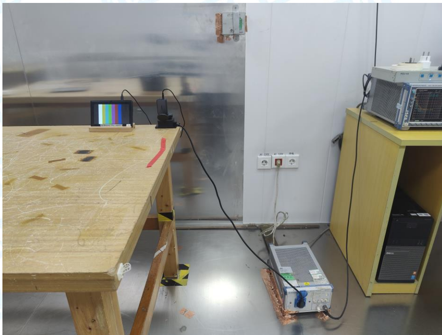
Photo of Setup for Conducted Emission
