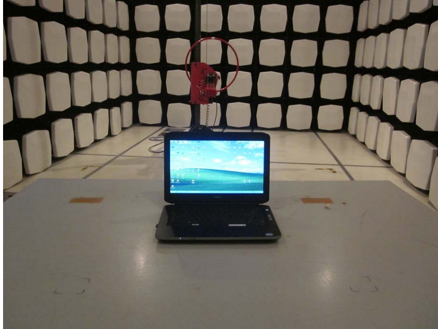
Measurement of Radiated Emission Test Set Up
