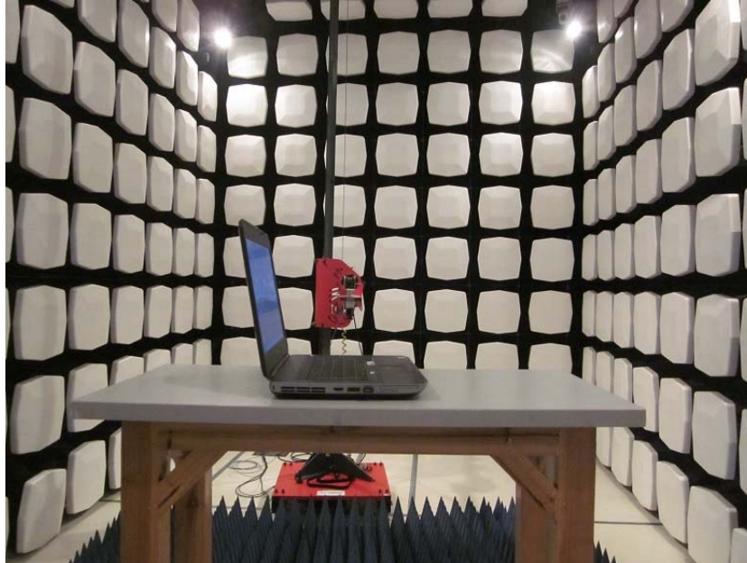
Measurement of Radiated Emission Test Set Up
