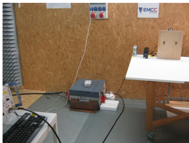
Conducted emissions measurement 150 kHz – 30 MHz
