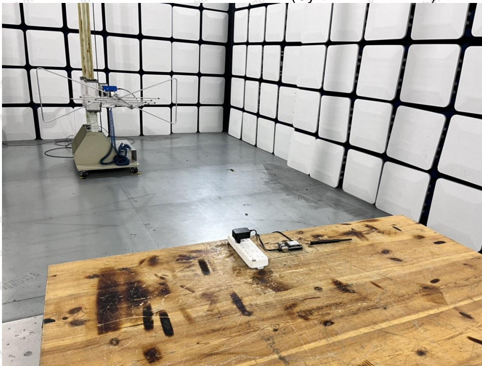
Photo of Radiation Emission Test (Cylindrical antenna)
