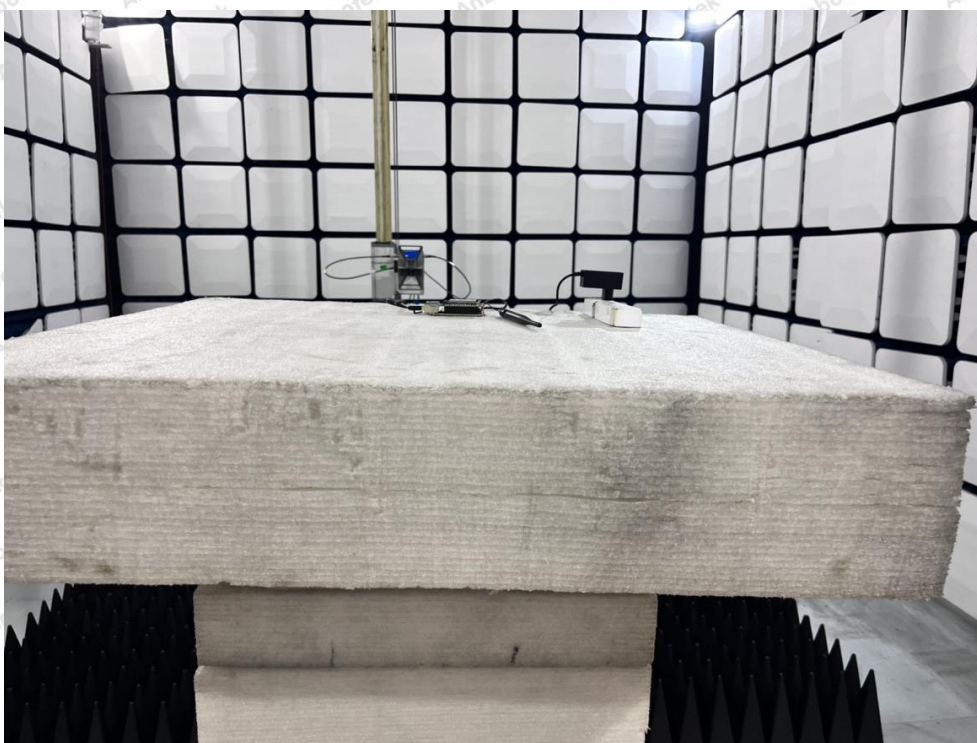
Photo of Radiation Emission Test (Sucker antenna)
