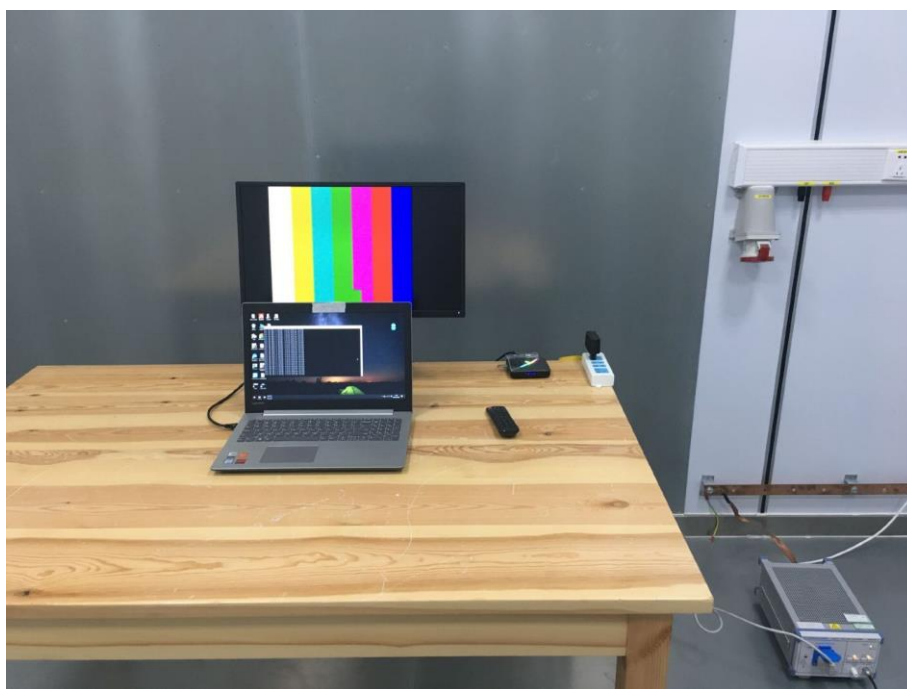
Fig. 4 Power line conducted emission setup photo
