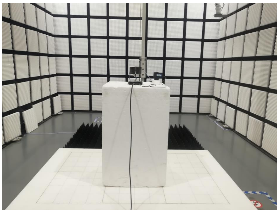
Fig. 3 Radiated emission setup photo(Above 1GHz)
