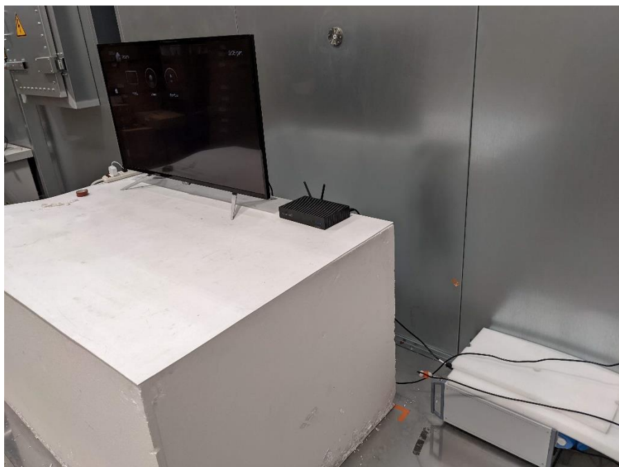
Photograph 5: Test Set Up AC Mains Conducted Emissions
