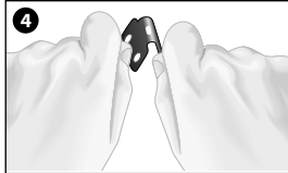
Bend bracket for correct detection angle (if needed).
