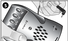
Plug power cord into detector.
