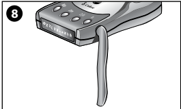
Place antenna facing towards dashboard if windshield angle prevents you from placing it upright.
