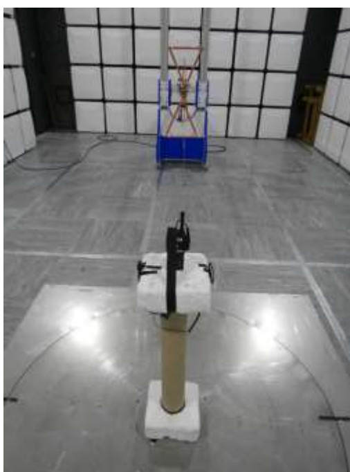
Figure 15 – Test Setup - 30 MHz to 1 GHz – Y Orientation
