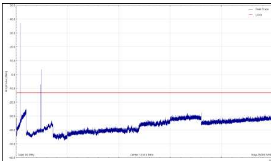
Figure 10 - 30 MHz to 25 GHz, Vertical – Y Orientation (ISED)
