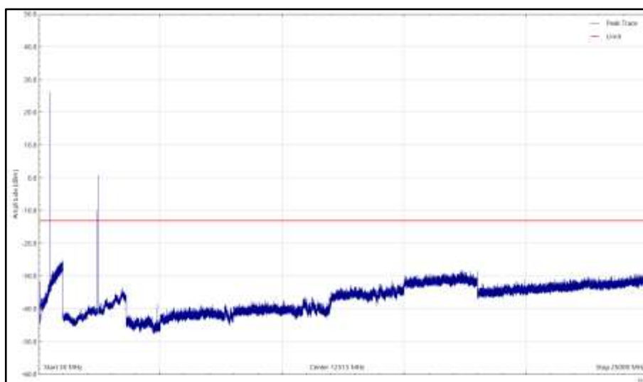
Figure 6 - 30 MHz to 25 GHz, Vertical – Z Orientation (FCC)
