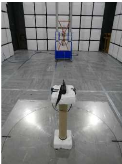
Figure 16 – Test Setup - 30 MHz to 1 GHz – Z Orientation
