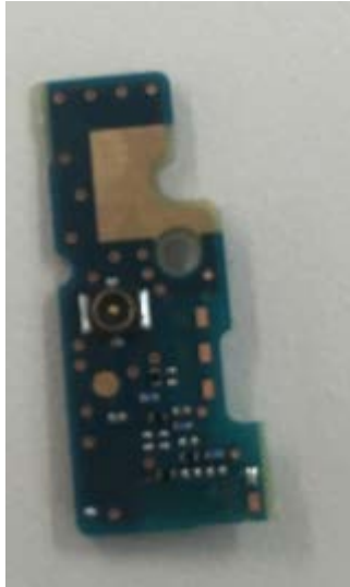
Internal Main_ANT-2-PWB (Front-side)
