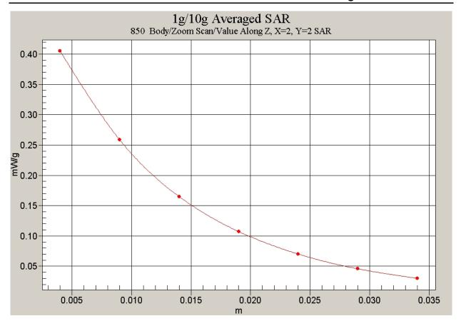
Fig. 28 Z-Scan at power reference point (Flat Phantom 850MHz CH190 with the display of the handset towards the ground)
