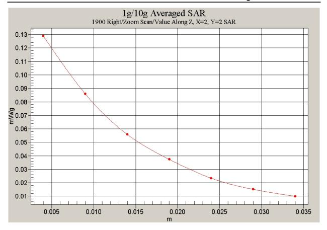
Fig. 50 Z-Scan at power reference point (Right Hand Tilt 15° 1900MHz CH810)
