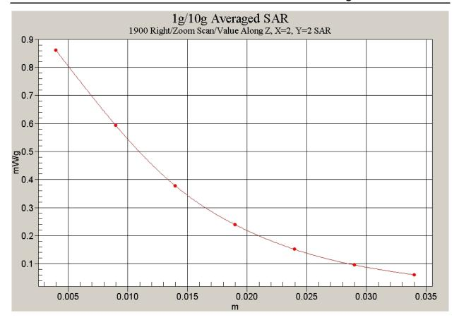
Fig. 44 Z-Scan at power reference point (Right Hand Touch Cheek 1900MHz CH810)
