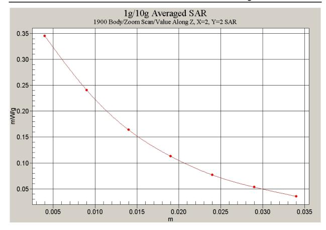
Fig. 56 Z-Scan at power reference point (Flat Phantom 1900MHz CH810 with the display of the handset towards the ground)
