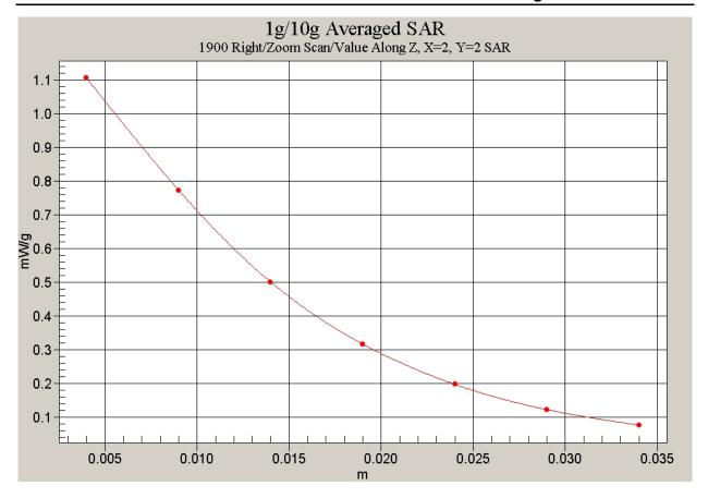
Fig. 48 Z-Scan at power reference point (Right Hand Touch Cheek 1900MHz CH512)
