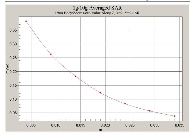
Fig. 58 Z-Scan at power reference point (Flat Phantom 1900MHz CH661 with the display of the handset towards the ground)
