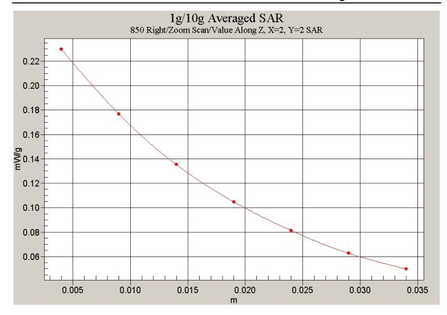
Fig. 24 Z-Scan at power reference point (Right Hand Tilt 15° 850MHz CH128)
