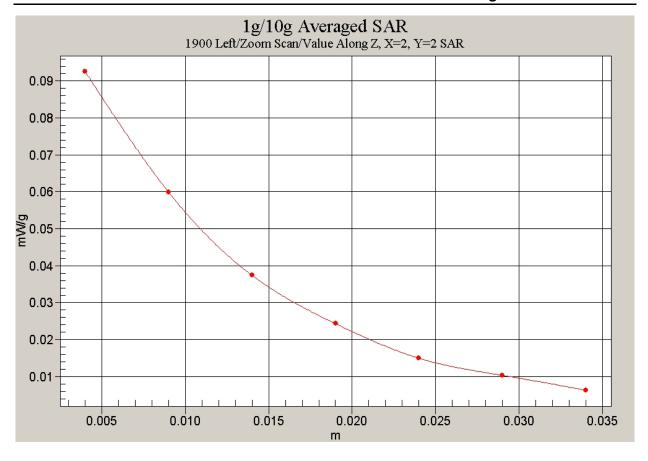
Fig. 38 Z-Scan at power reference point (Left Hand Tilt 15° 1900MHz CH810)
