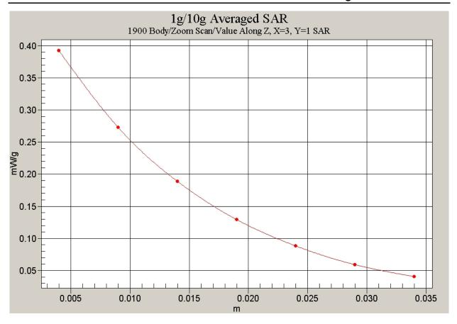
Fig. 60 Z-Scan at power reference point (Flat Phantom 1900MHz CH512 with the display of the handset towards the ground)
