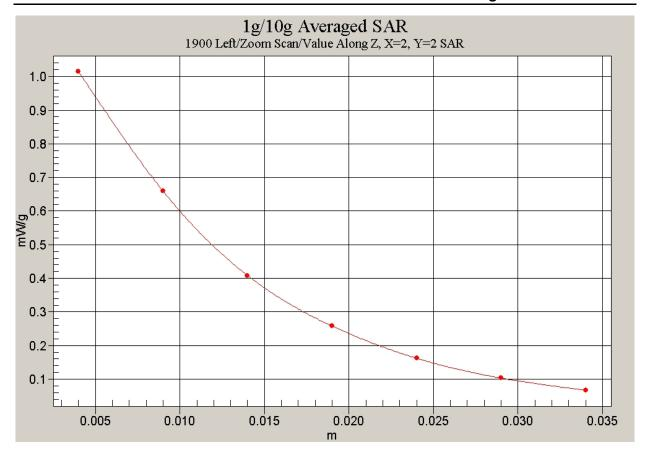
Fig. 36 Z-Scan at power reference point (Left Hand Touch Cheek 1900MHz CH512)
