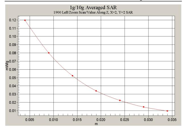
Fig.42 Z-Scan at power reference point (Left Hand Tilt 15° 1900MHz CH512)
