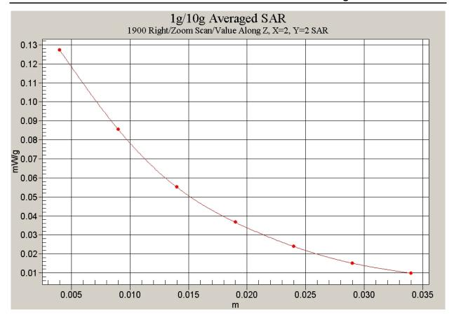
Fig. 54 Z-Scan at power reference point (Right Hand Tilt 15° 1900MHz CH512)
