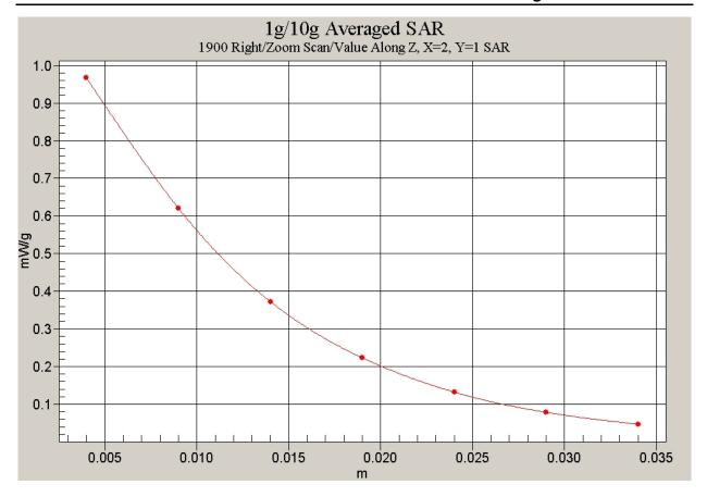
Fig. 46 Z-Scan at power reference point (Right Hand Touch Cheek 1900MHz CH661)
