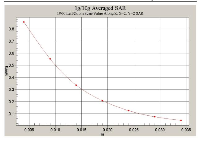
Fig. 34 Z-Scan at power reference point (Left Hand Touch Cheek 1900MHz CH661)
