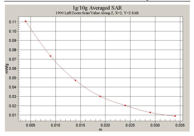
Fig. 40 Z-Scan at power reference point (Left Hand Tilt 15° 1900MHz CH661)
