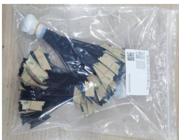
Figure 1: A bundle of terminal heads is wrapped with foam and put into PE bags, each bag 200/PCS
