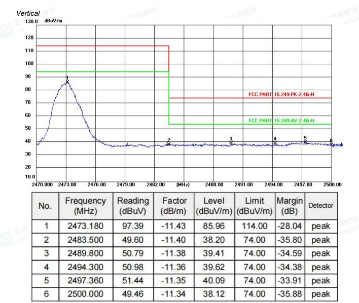
Note: Due to the measure PK emission level less than the AV limit value. No necessary to take down the AV emission level.
