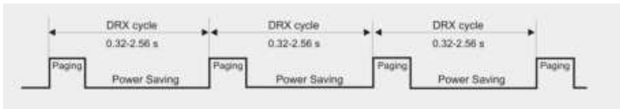
Figure 38: Power saving and paging in LTE networks
