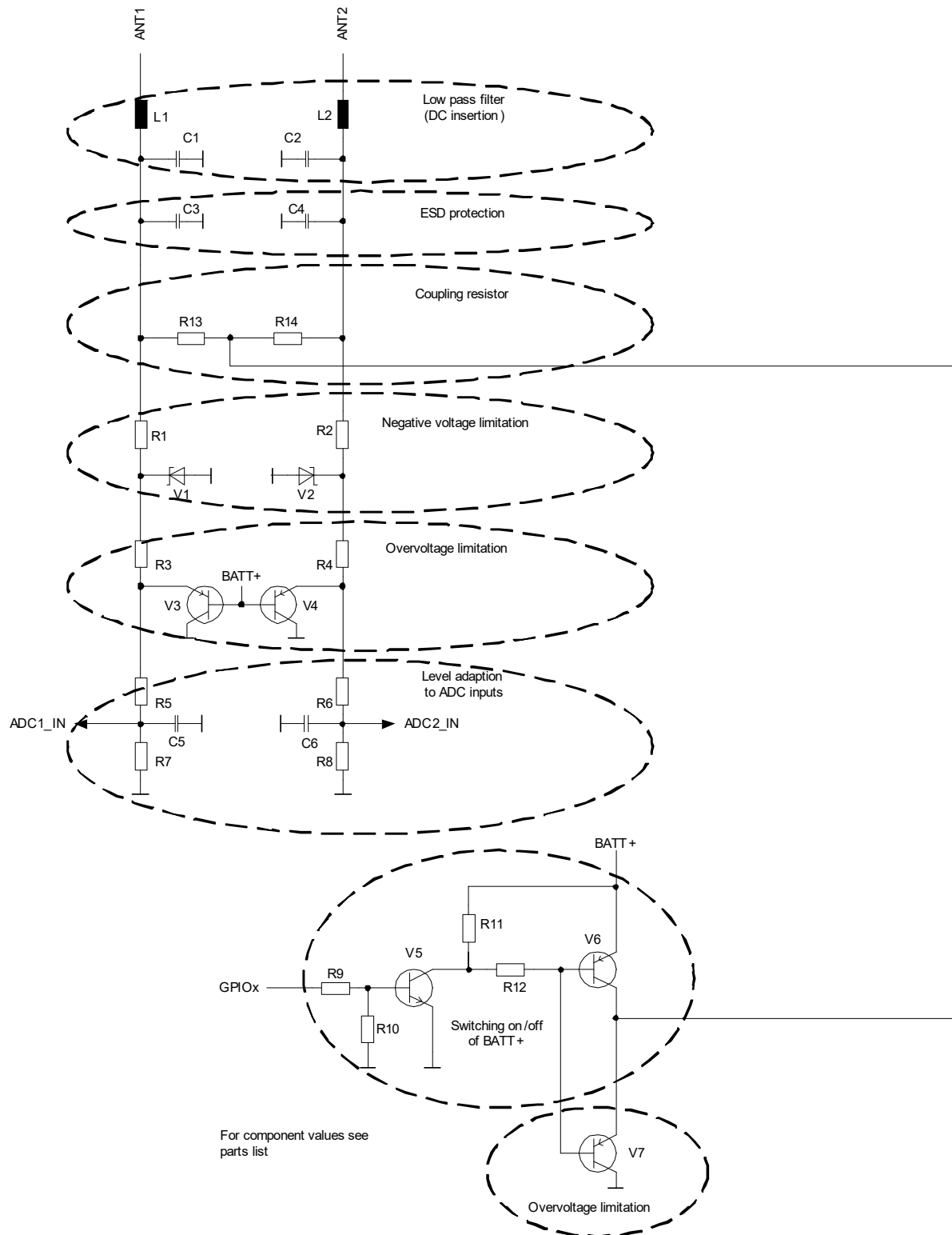
Figure 29: Antenna detection circuit sample - Schematic
