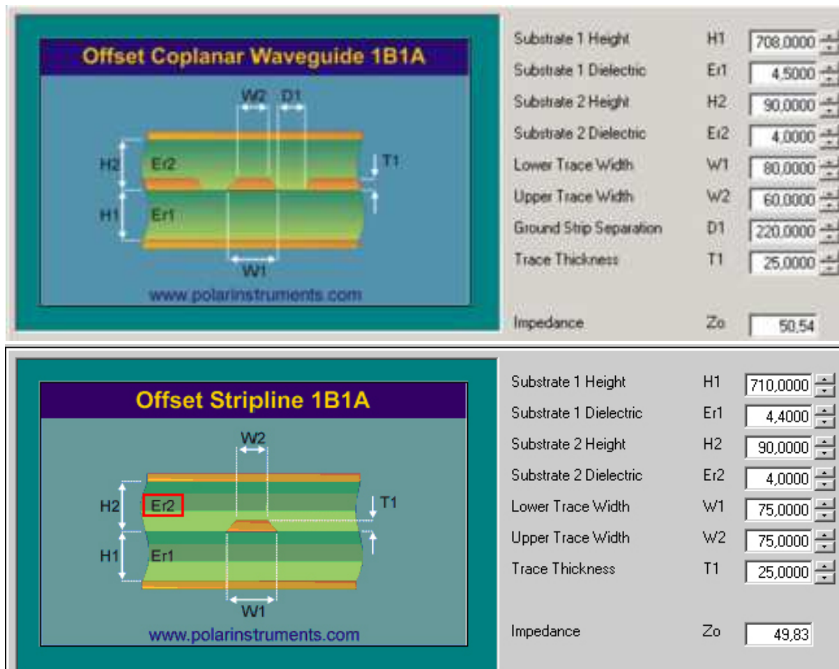
Figure 18: Embedded Stripline line arrangement
