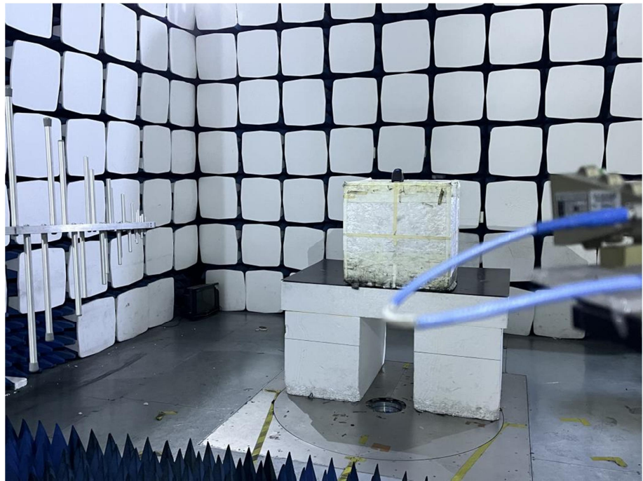
Radiation Emission Test Setup (Above 18GHz)
