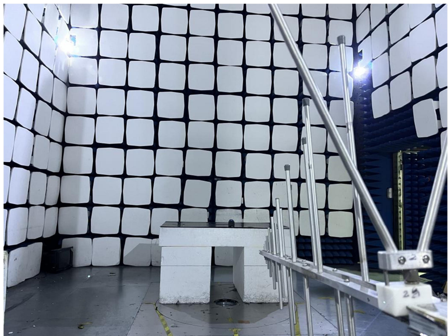
Radiation Emission Test Setup (30MHz to 1GHz)
