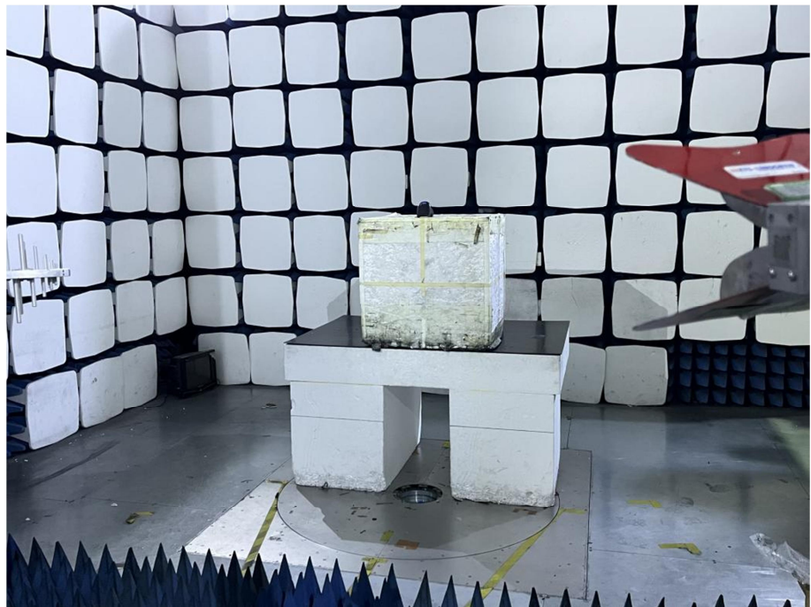
Radiation Emission Test Setup (1GHz to 18GHz)
