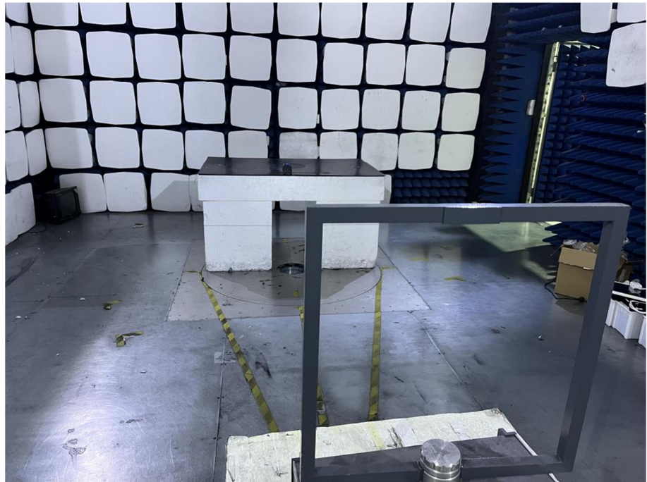
Radiation Emission Test Setup (Below 30MHz)
